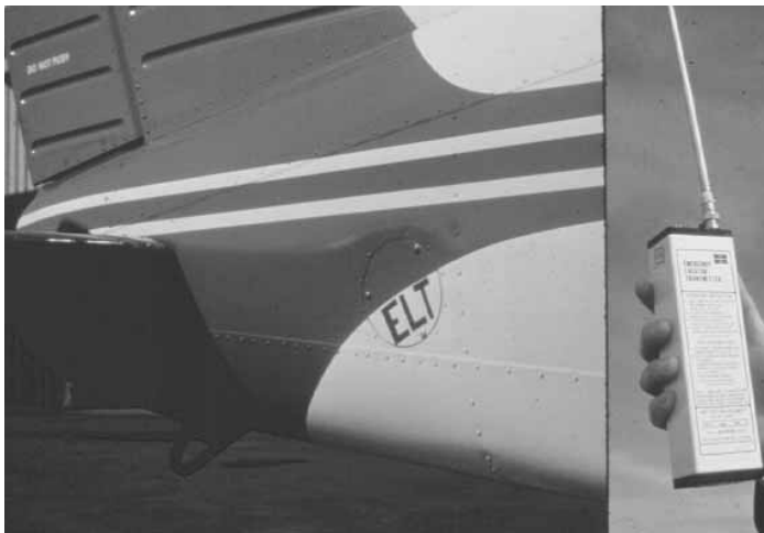
121.5 MHz emergency locator transmitters were installed on small aircraft.
