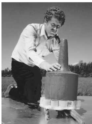
Tests of a maritime beacon through a satellite are conducted.
