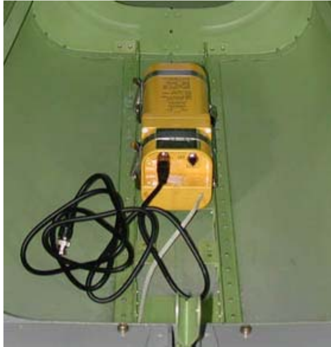
Figure 3: ELT securely mounted to aircraft frame
