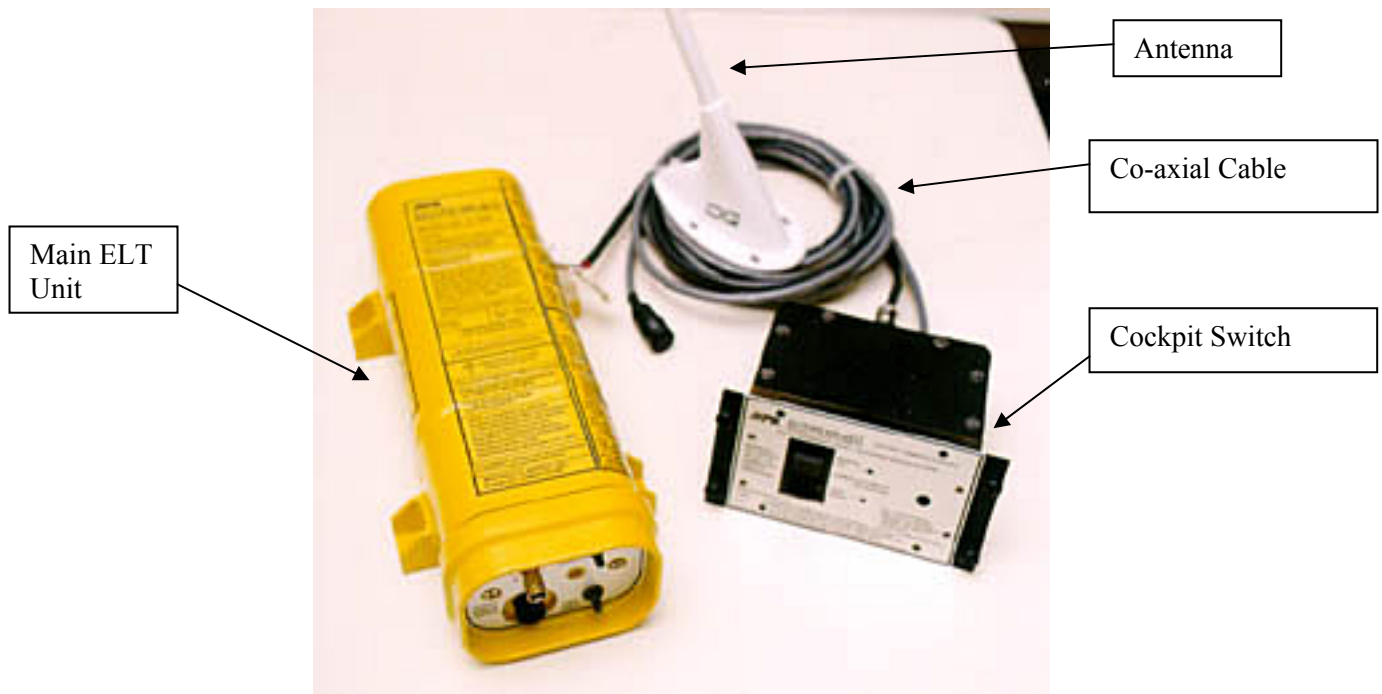
Figure 2: Main components of an ELT. Image from Transport Canada - as part of a National SAR Secretariat New SAR Initiative sponsored project in 2006. http://www.tc.gc.ca/innovation/tdc/projects/air/e/8030.htm
